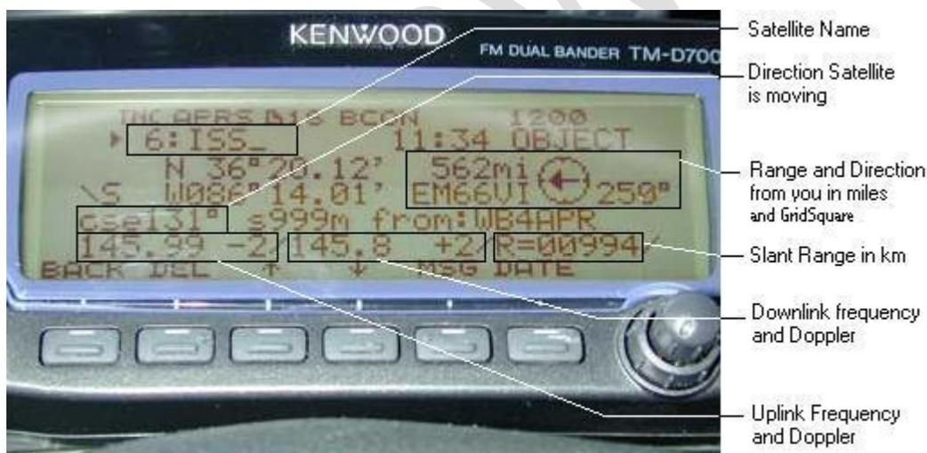
D-700 Front Panel Display of Satellite-in-view
