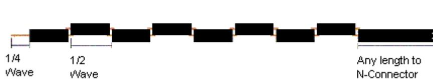
$$1/2 \text{ 波长} = \frac{V * C}{2 * F} = \frac{0.66 * 299792458}{2 * 2441000000} = 0.0405\text{m} = 40.5\text{mm}$$
